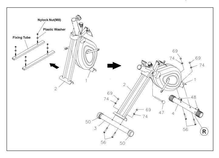
NOTE: Remove the FIXING TUBES, WASHERS, and NUTS from MAIN FRAME(1) and REAR FRAME(2) before any assembly. These parts are only for packing, do not dispose of the packing materials until assembly is completed.
